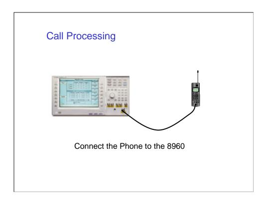
Begin by connecting the phone to the 8960. The phone has an antenna RF In/Out connector which must be connected to the 8960 RF In/Out connector. The GSM phone should be supplied with the RF Interface cable.
