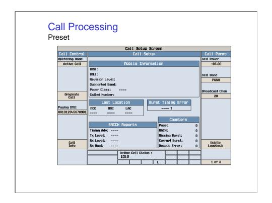
Begin the test procedure by resetting the instrument. Press the blue 'SHIFT' button then the RESET button.
