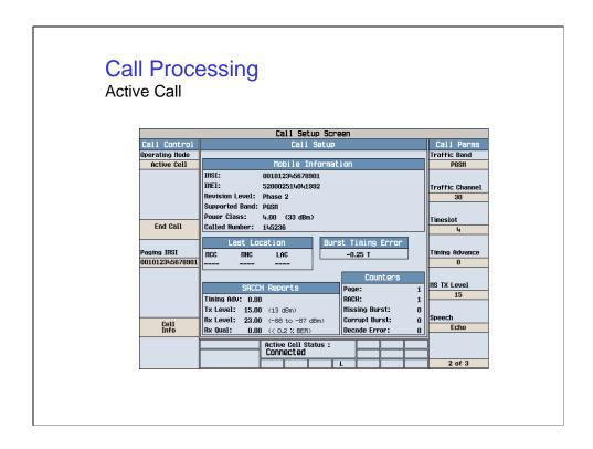
When a call is connected the test data should appear in the 'Burst Timing Error' window and in the 'SACCH Reports' window, the 'Active Cell Status' window should say 'Connected'. Disconnect the call by pressing the 'End Call' button on either the phone or the 8960.
