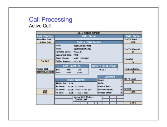
When a call is connected the test data should appear in the 'Burst Timing Error' window and in the 'SACCH Reports' window, the 'Active Cell Status' window should say 'Connected'. Do not disconnect, proceed to the next tests.
